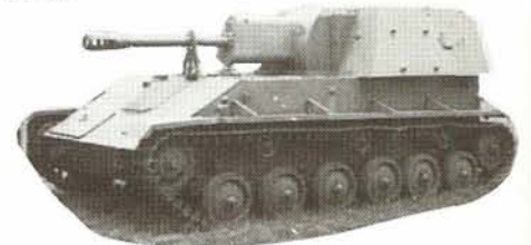
SU-76 — the first Soviet assault gun mounting a 76.2mm gun, L/41.5.
